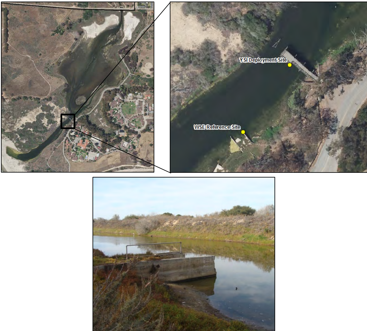
Figure 1. Map showing the location where the YSI EXO-1 data sonde is installed on the “pier” in the main channel of Devereux Slough, and the location of the elevation benchmark atop the concrete wall with staff gauge (also in photo), where the reference water surface elevation (WSE) is manually measured in order to adjust the sonde water level data to WSE in feet (NAVD).
